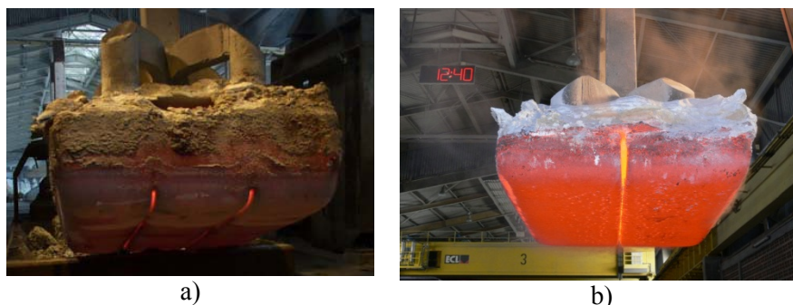
Figure 3. Slotted (a) and shape modified anode (b).
